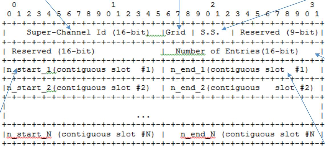
Number of 32-bit entries in the super-channel label, where each entry is a contiguous slot of optical spectrum
