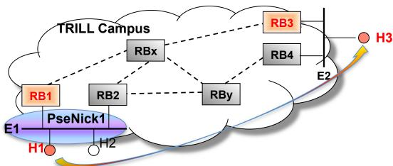
When RB1 encapsulates H1's native data frame into TRILL form, the ingress nickname in TRILL header is PseNick1 not RB1 if the pseudonode nickname function is enabled on link E1
