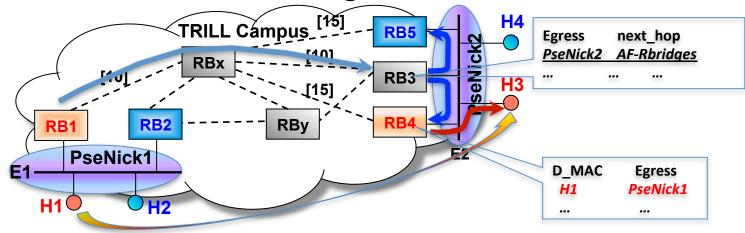
The forwarding remains unchanged in form, but a multicast MAC, i.e., "AF RBridges on this link" is required
