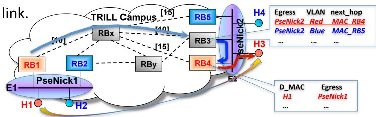
In this approach, the forwarding table has to be based on {nickname, VLAN}, instead of {nickname}, because RB3 must know which Rbridges on E2 is VLAN-Red AF just from the view of data plane
