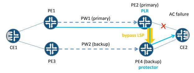
PE4 (protector PE) sends packets to CE2 based on PW label (i.e. upstream label) assigned by PE2.
