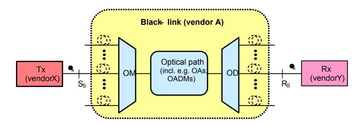
**Black Link:** The Black Link approach [ITU-T G.698.2] allows supporting an optical transmitter/receiver pair of one or different vendors to inject an Optical Channel (OCh) and transfer it over a DWDM network composed of amplifiers and add-drop multiplexers from a different vendor. Therefore the standard defines the ingress and egress parameters at the reference points Ss and Rs.
