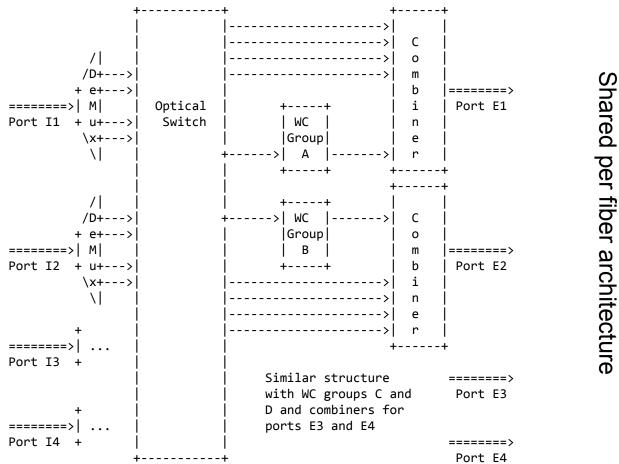
Numbers: 4 ports, 200 wavelength converters, 10 types of converters, random assignment of converters to groups.
