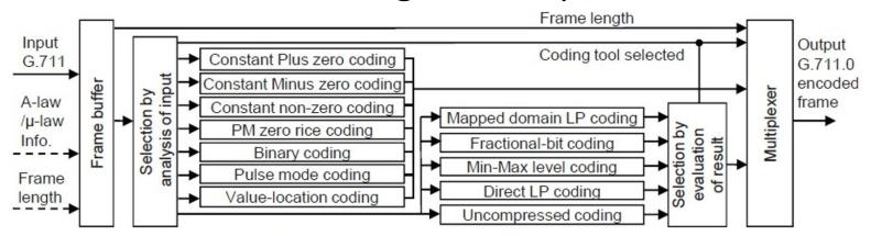
Fig. 1. High-level block diagram of the G.711.0 encoder.
