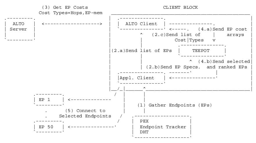
Figure 2: Multi-Cost ALTO scenario and transactions in a client block
