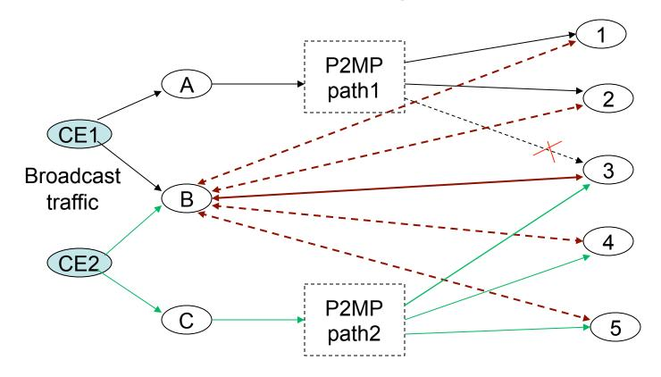
when Node B received the extensive APS or PSC Message, it will send the service packet of selected protected working path by p2p protecting Tunnel(B-3). For other leaf node 1 and 2 still receive service packet from working path 1
