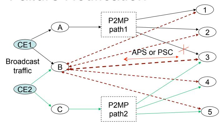
when leaf node 3 detects a defect on the branch path(A-3). Leaf Node 3 would select one path to be protected based on the priority, then switch to the protecting path to receive the service packet and send extensive APS or PSC message including the selected defective working path ID to source protection node B by p2p tunnel;
