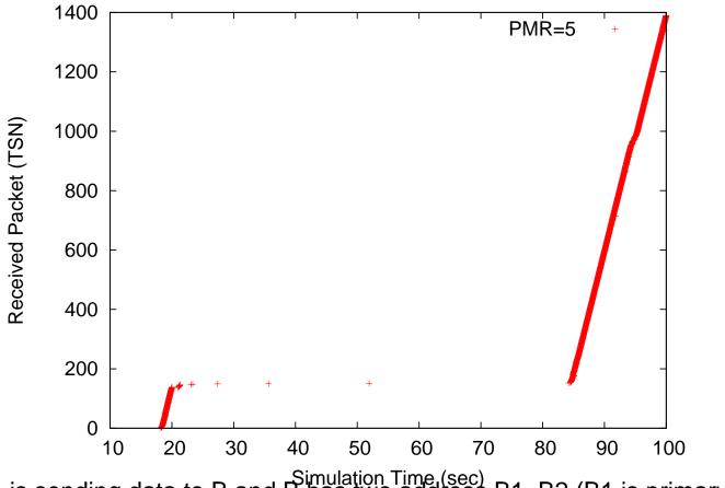
A is sending data to B and B has two address B1, B2 (B1 is primary) when primary becomes unavailable at 20 sec, it takes 60 secs to restart data transmission. (Path.Max.Retrans = 5)
