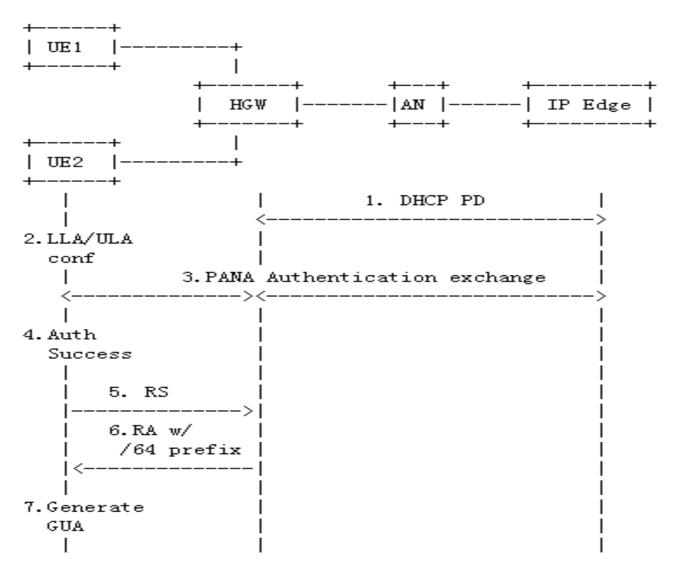
Figure 1: IPv6 Broadband Access Network
