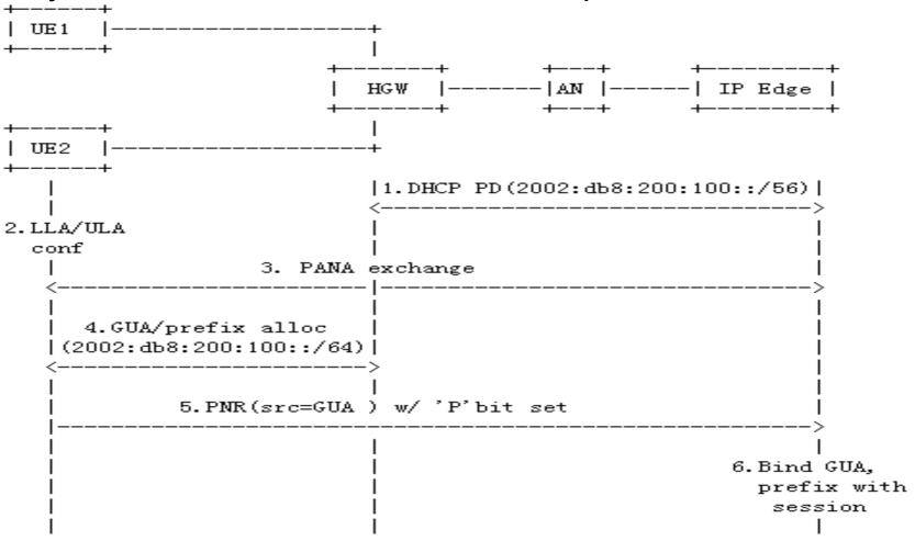
Figure 3: Message flow of IP/prefix reconfiguration in home network -2
