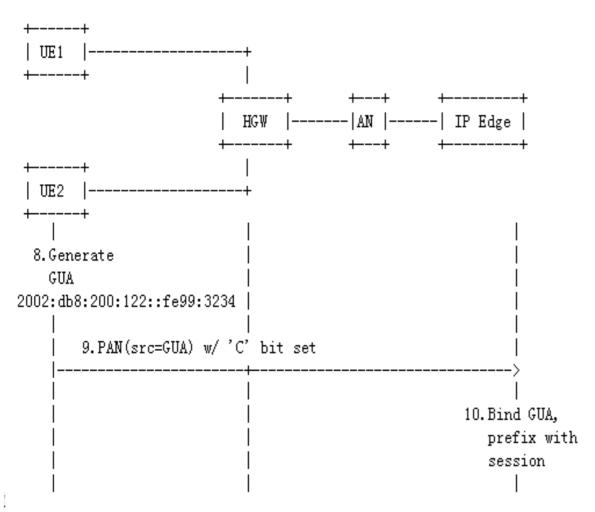
Figure 2: Message flow of IP/prefix reconfiguration in home network -1
