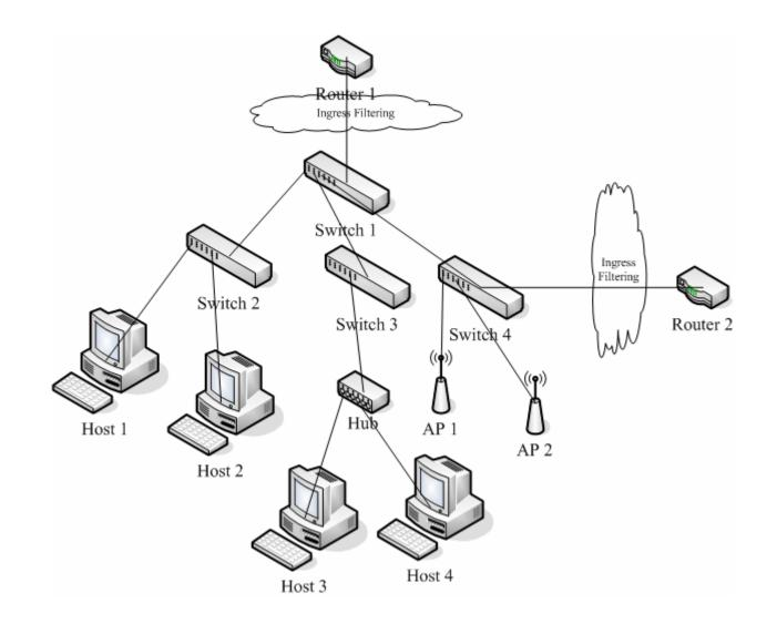
Figure 1 Typical SAVI access network
