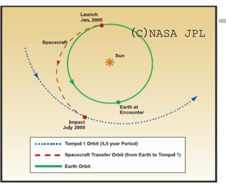
Traveling at a relative velocity of 10 km/s and from about 864,000 km (536,865 miles) away, the impactor must strike the 6 km (3.7 mile) diameter comet.
