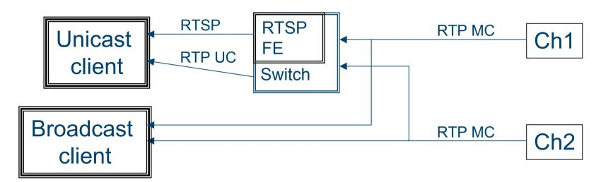
Both clients can view the same channels. For the unicast client RTSP is used to control the streams.
