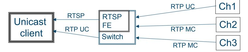
RTSP is used to control the RTP unicast sessions between client and server (switch)
