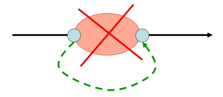
The repairing router delivers the packet downstream of the failure, NOTVIA the failure.
