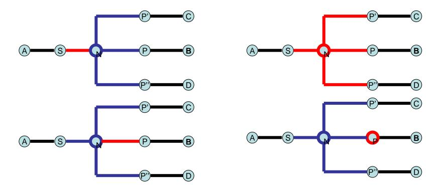
Without further diagnostics, it does not know whether its connection to the LAN, P's connection to the LAN, the LAN, or P has failed.
