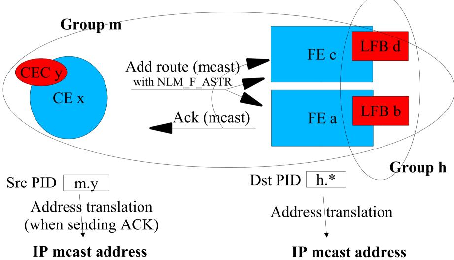
IP mcast address containing CE x, FE c and FE a.
