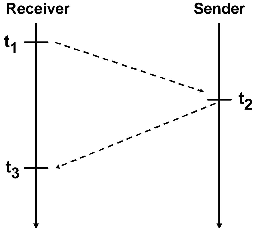
Upper bound on sender's time:  $t_S < t_R - t_1 + t_2$
