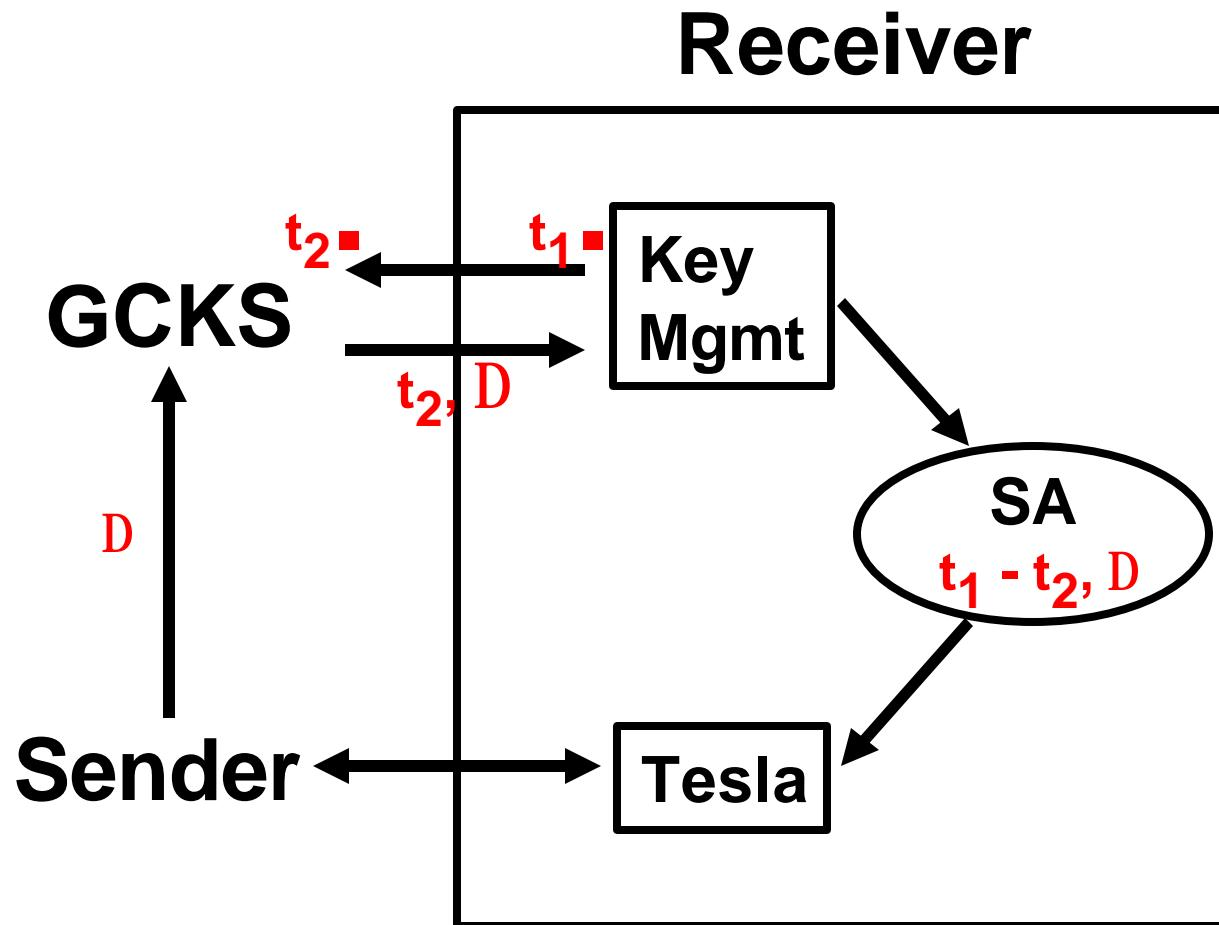
Upper bound on sender's time:  $t_S < t_R - t_1 + t_2 + D$
