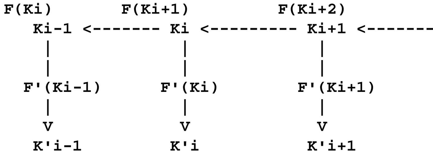
Based on an old scheme: Lamport's One-Way Hash Chain (1981) and S/KEY (RFC 1760). HMAC-SHA1 is just one type of one-way function that can be used.
