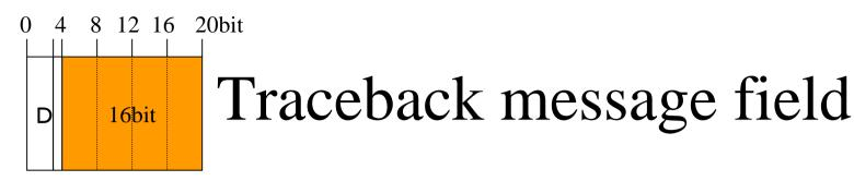
Traceback message field is using for sending a passing router infomation to destination node.
