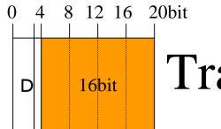
Traceback message field is using for sending a passing router infomation to destination node.
