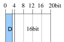
Distance field indicates hop counts from first marked router and is increased by each passing routers.
