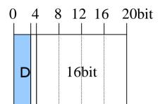
Distance field indicates hop counts from first marked router and is increased by each passing routers.
