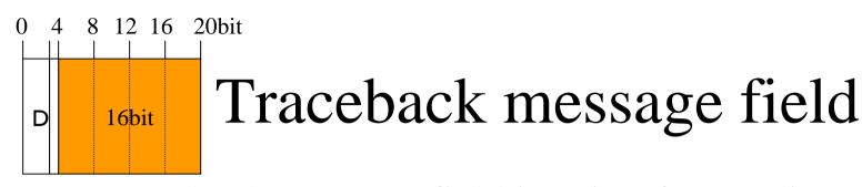
Traceback message field is using for sending a passing router infomation to destination node.
