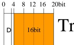
Traceback message field is using for sending a passing router infomation to destination node.
