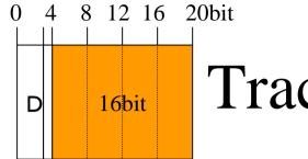
Traceback message field is using for sending a passing router infomation to destination node.
