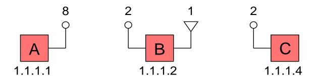
Node **A** communicates with **C** using source route  $1.1.1.1/8 \rightarrow 1.1.1.2/2 \rightarrow 1.1.1.4$
