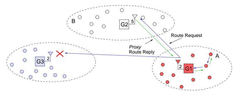
**Proxy** reply mechanism can localize topological change
