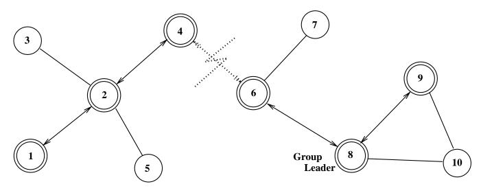
Node 4 detects link breakage, initiates group repair
