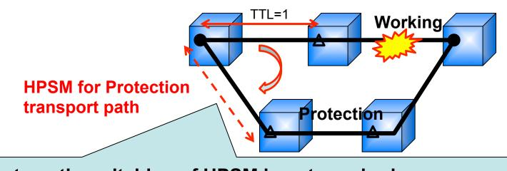
Automatic switching of HPSM is not required (TTL re-discovery is not required in case of protection SW)
