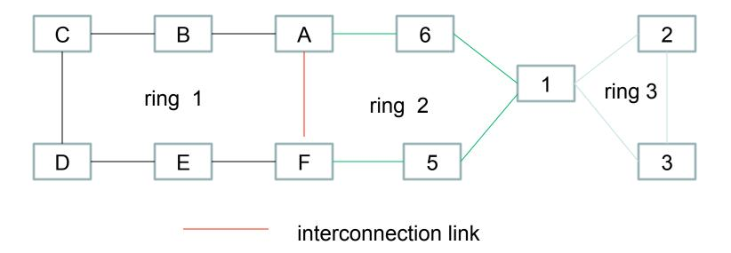
For the mixed interconnection, it may separately use recovery mechanism of single-node or chained interconnection to recovery the failure between any two directly connected-ring. In addition, it still may set up end to end protection path which traverse ring 1,ring 2 and ring 3 to recovery the multi-ring service.
