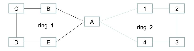
As the interconnection node( eg. Node A ) is only a single point that connect two ring , when the failure happens on the interconnection node, the multi-ring service may not be recovery, so the scenario should be avoided.
