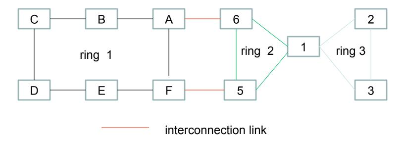
For the mixed interconnection, it may separately use recovery mechanism of dual-node or single-node interconnection to recovery the failure between any two directly connected-ring. In addition, it still may set up end to end protection path which traverse ring 1,ring 2 and ring 3 to recovery the multi-ring service.
