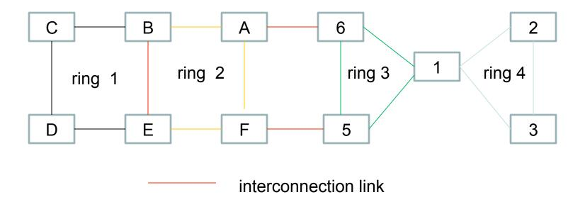
For the mixed interconnection, it may separately use recovery mechanism of dual-node or chained ,single-node interconnection to recovery the failure between any two directly connected-ring. In addition, it still may set up end to end protection path which traverse ring 1,ring 2, ring 3 and ring 4 to recovery the multi-ring service.
