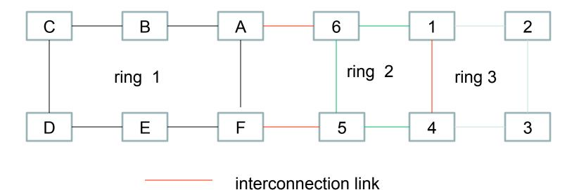
• For the mixed interconnection, it may separately use recovery mechanism of dual-node or chained interconnection to recovery the failure between any two directly connected-ring. In addition, it still may set up end to end protection path which traverse ring 1,ring 2 and ring 3 to recovery the multi-ring service.
