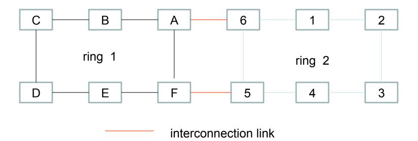
• For the interconnection scenario, it may use 1:1 linear protection to recovery the failure of interconnection link. In addition, it still may set up end to end protection path which traverse ring 1 and ring 2 to recovery the multi-ring service;
