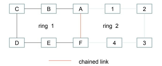
For the interconnection scenario, when interconnection node( node A or node F) or link(A-F) has the failure, it may set up end to end protection path which traverse ring 1 and ring 2 to recovery the multi-ring service.
