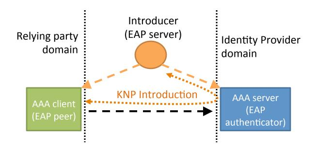
When an AAA Client and a AAA Server are connected via a single KNP Introducer, this is referred to as a Trust Link
