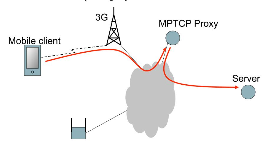
MPTCP client sends SYN to proxy, indicating address of final server. Proxy initiates connection to server.
