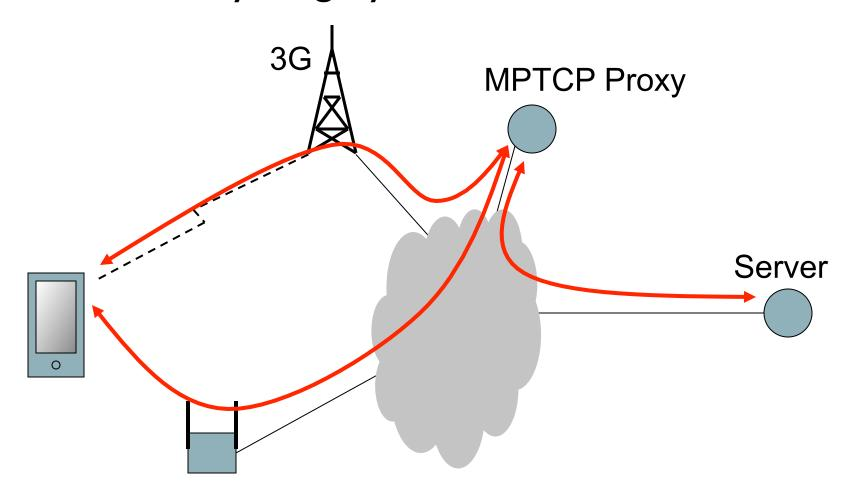
New subflows are set up to the proxy, which load-balances in the normal MPTCP manner.
