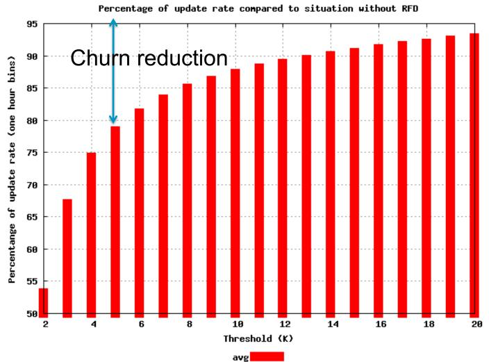
Update rate is reduced by more than 20 % with [4K-5K], compared to no suppress threshold
