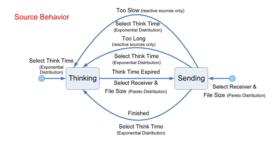
For simplicity, the state diagram omits a flow connection phase that occurs prior to sending, and also the potential for connection failure after which a source reenters the thinking state
