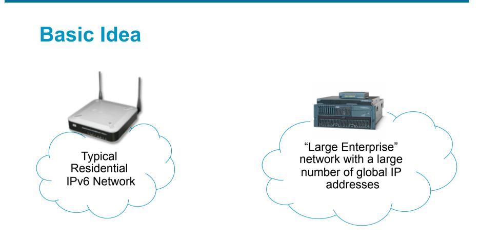
Observation: Expansive addressing in IPv6 allows any residential network to resemble an enterprise network with a large IPv4 global address block
