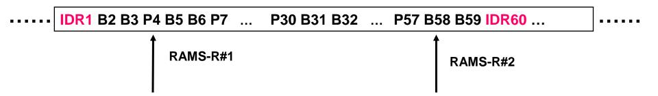
If the RR starts to request the acquisition close to the next random access point (RAP), e.g. RAMS-R#2 above, the acquisition delay will be lower if the receiver had chosen to directly join the multicast group.
