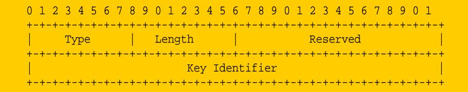
**Key (4 octet)-** assigned in the Registration and inserted in every GRE frame. Value to be assigned by IANA.
