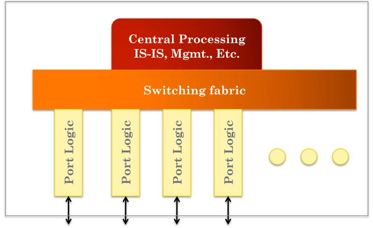
Links to other devices. Could be 802.3 (Ethernet), 802.11 (Wi-Fi), PPP, ...
