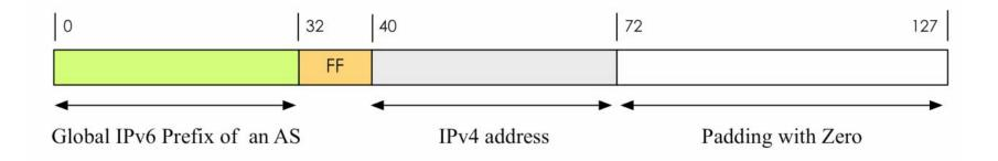
Mapping Rule: IPv4 addresses are embedded from bit 40 to bit 72 of the IPv6 addresses of a specific /32.
