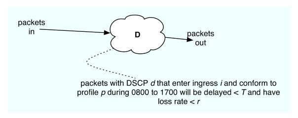
Outcome: **for** a traffic stream within particular rate bounds and temporal characteristics and (optionally) on the correct interface and with the correct markings, **get** certain service characteristics (loss rate, delay bound, etc) across the network domain.
