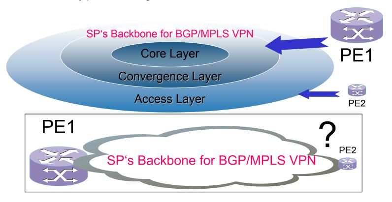
PE1 and PE2 should maintain the same VPN routes. However, if VPN route table is large, PE2 will have capacity and performance issues.
