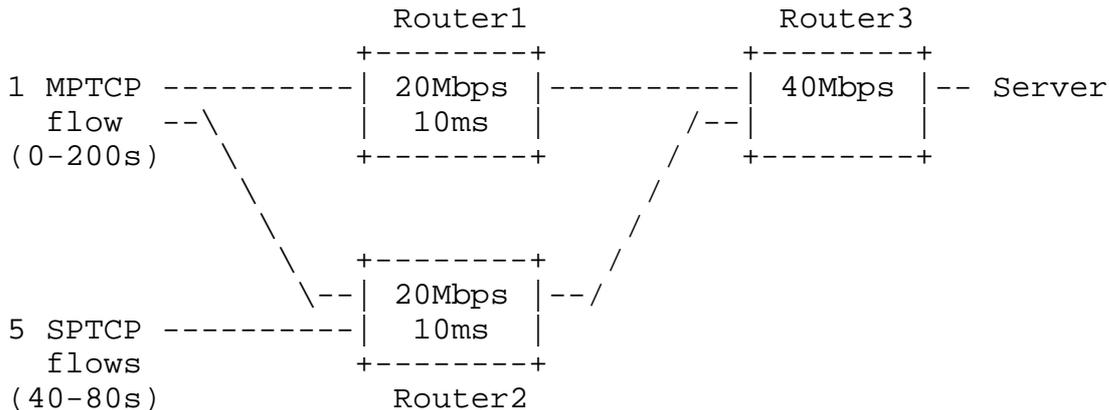
Figure 2: Testbed topology for the responsiveness scenario.
