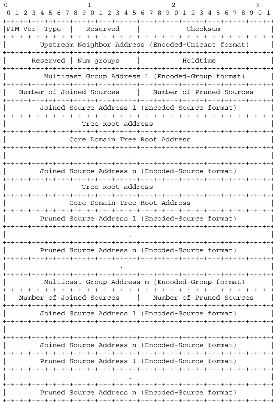
Figure 10 Join/prune message format
