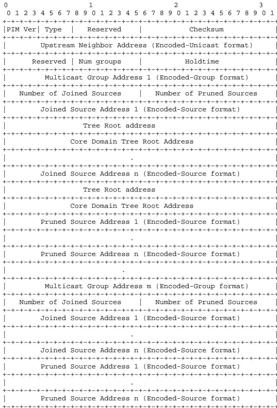
Figure 10 Join/prune message format
