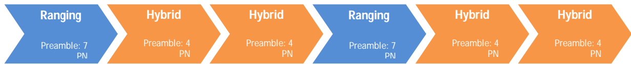
Figure 6: Optional slot structure for a given transmitter. The blocks above are 1 or more sec apart and represent 1 slot (100ms). The lengths of the preamble, pilot, and data portions in the above diagram correspond to the sample scenario where m=2, n=1 and where there are two hybrid slots for each ranging slot.
