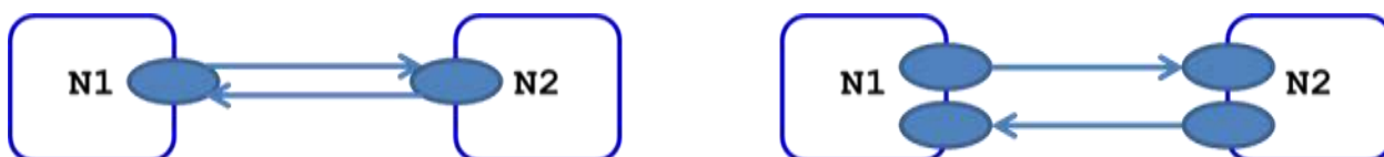
Figure 2a. Bi-directional TE link combination (left), independent uni-directional TE links (right)
