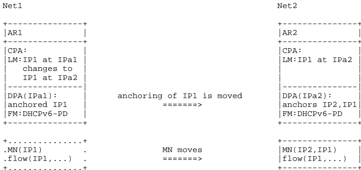
Figure 8. IP prefix/address anchor switching to the new network. MN with flow using IP1 in Net1 continues to run the flow using IP1 as it moves to Net2.
