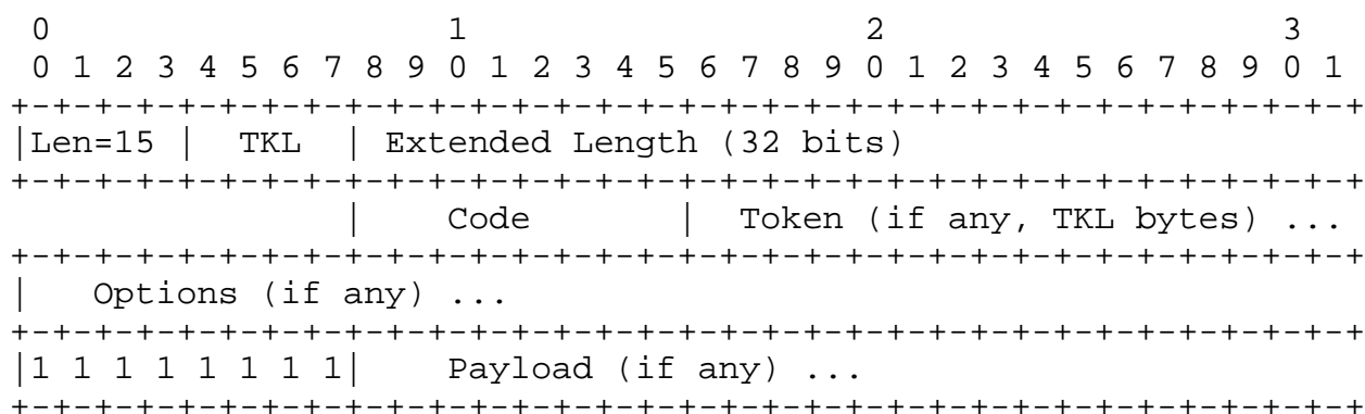
Figure 8: CoAP message format with 32-bit Extended Length field
