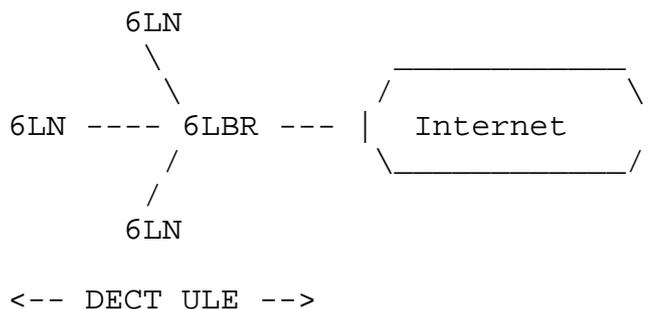
Figure 5: DECT ULE network connected to the Internet
