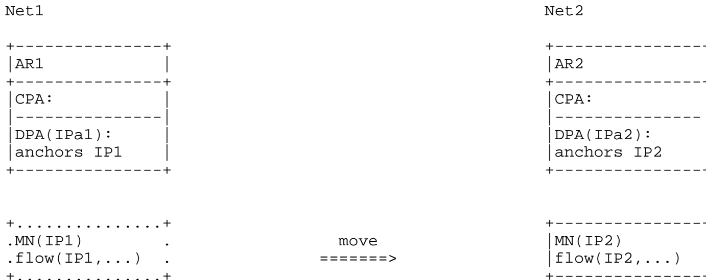
Figure 3. Changing to the new IP prefix/address. MN running a flow using IP1 in Net1 changes to running a flow using IP2 in Net2.
