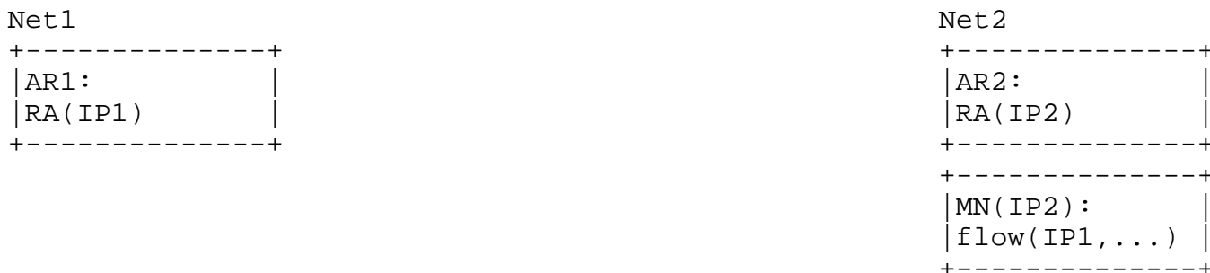
Figure 4. IP address anchored not in network of attachment. MN attached to AR2 in Net2 has a flow(IP1,...) using IP1, which belongs to Net1.
